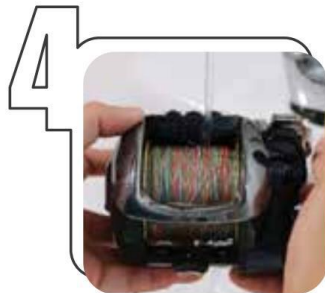
Rinse the spool area for removal of remaining salt
