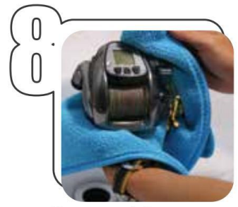
Use a wet cloth to wipe down the whole reel to ensure remaining salt and bait is removed
