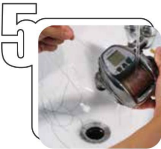
Engage clutch and pull out 2-3 meter of line while running low pressure water
