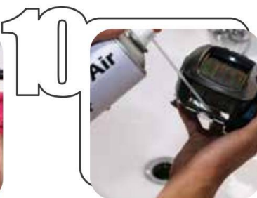
Use an air duster to spray difficult access area to clear off water droplets
