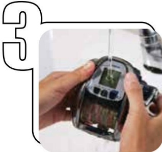
Quick run through of low pressure water on screen (not more than 3 seconds)
